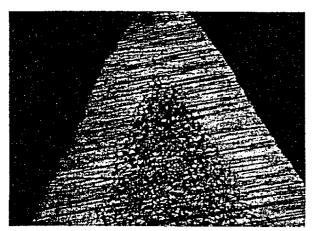
125/140 µm Case Depth - Water Quench from 775°C Magnification of 100X, Nital Etch.
